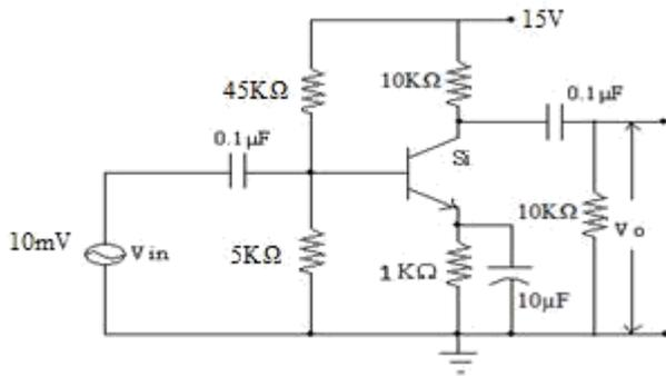
28. Determine the output voltage, when  $V_i = 5 \sin 100\pi t$
